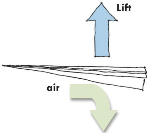
As a paper aeroplane moves forward, its wings push air down and this is what creates lift. By Newton's third law of motion (which states that every action has a reaction that is opposite and equal) pushing the air down has the effect of pushing the plane up.
